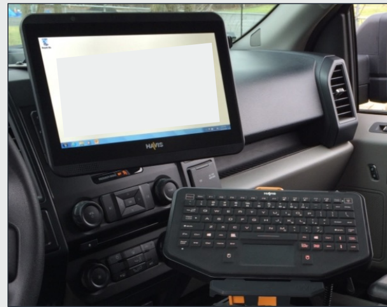
CLOSE TO DASH SCREEN MOUNT SYSTEM WITH LAPTOP MOUNTED IN TRUNK
